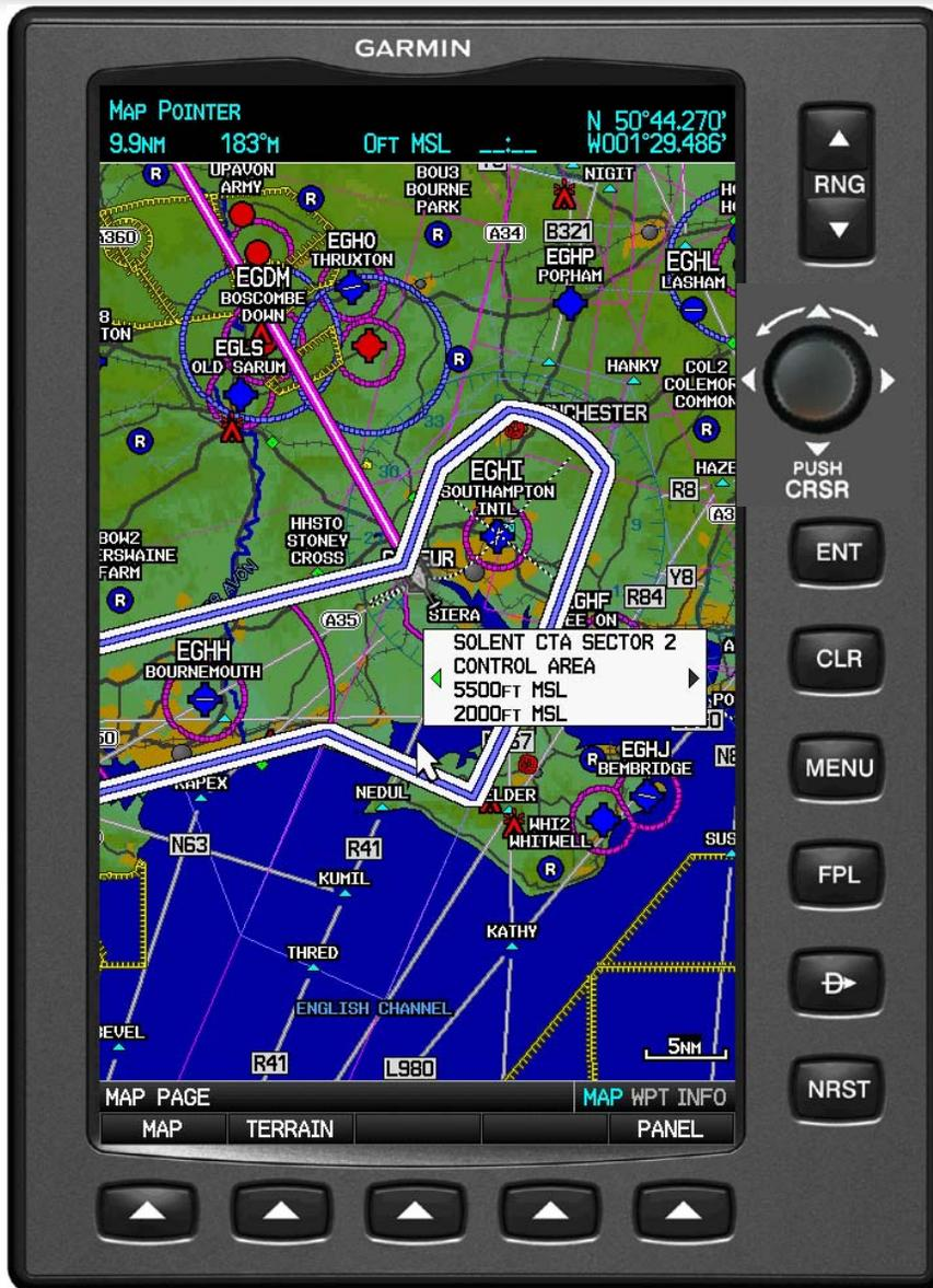
Easy access to layered map information. When panning the map, if multiple airspace/other data is available under the cursor, twisting the knob lets you easily access all data available under the cursor one at a time.
