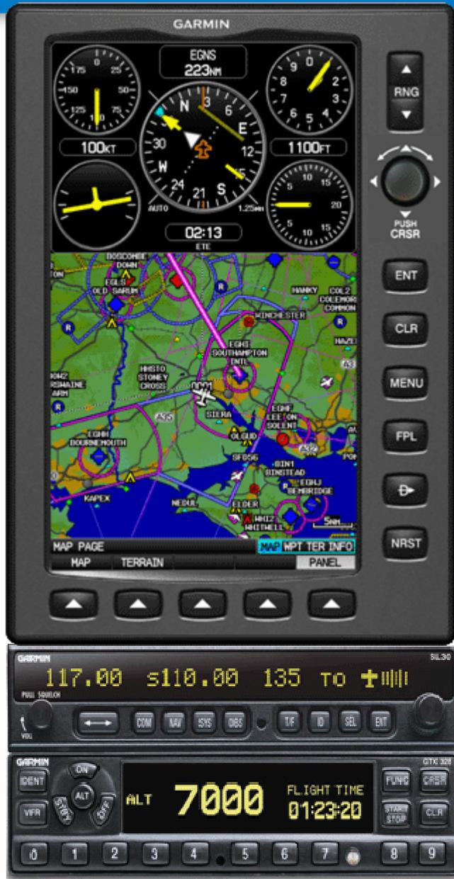
The GPSMAP 695 can be stacked together With the SL30/40 for transfer of frequency data for active waypoints (airports) or Navaids
