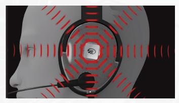
**Streaming Quiet™ ANR** allows Zulu PFX to adapt to your environment. Streaming Quiet uses ambient microphones to *continuously* sample cockpit noise before it penetrates the ear cup. An internal microphone placed near the ear canal monitors ANR performance.
